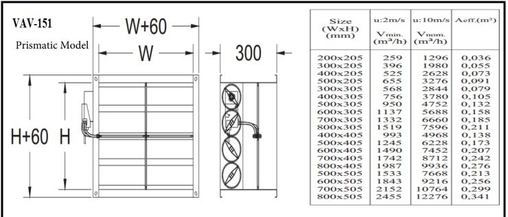
V<sub>min.</sub>(m³/h): Air flow rate when air velocity is 2 m/s V<sub>nom.</sub>(m³/h): Air flow rate when air velocity is 10 m/s V<sub>max.</sub>(m³/h): Air flow rate that customer wants between
